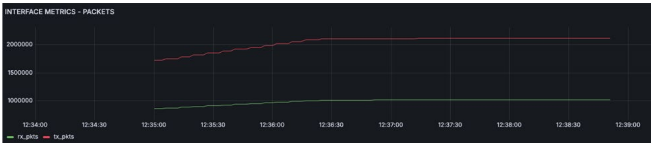
Figure 6 Total number of RX and TX packets processed by the NetScaler CPX interface over time
