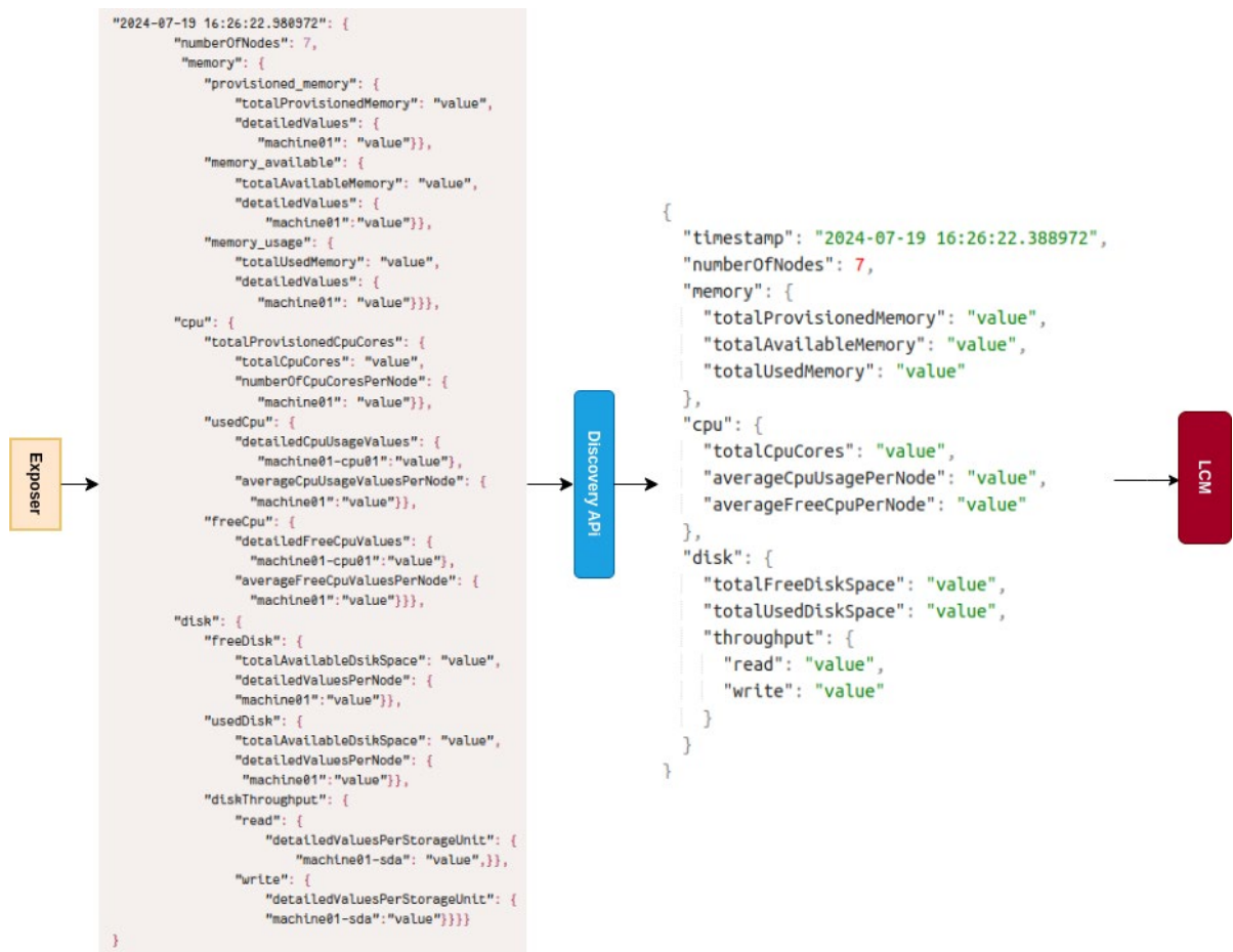
Figure 14 Aggregation and abstraction of resource metrics by Discovery for the LCM.
