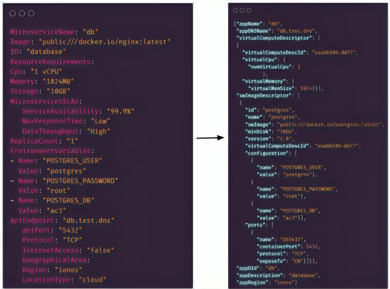
Figure 8: mapping between one of the use case 2 microservices configuration in the App Descriptor to its equivalent in the NSD format
